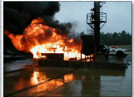
Testing configuration NHTSC burn evaluation for transport casks
