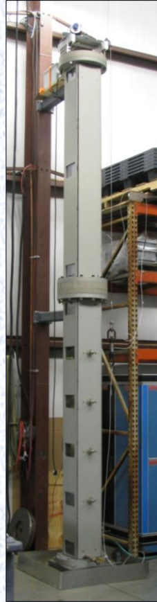
Testing configuration for distortion of nuclear fuel assemblies during operation
